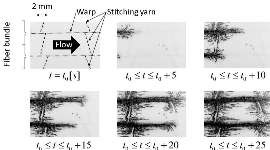
**Figure 1:** Progress of trajectories of particles suspended in epoxy under pressure difference  $\Delta P = -90$  kPa.
